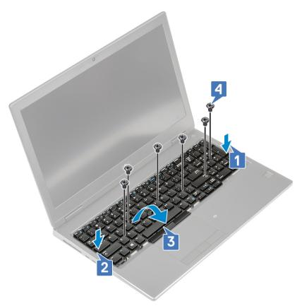
d Align the keyboard lattice to its position on the keyboard and ensure that the keyboard lattice clicks into its place.
