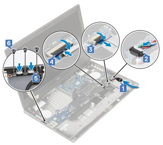
f Connect the power connector cable to the connector on the system board [1, 2].
