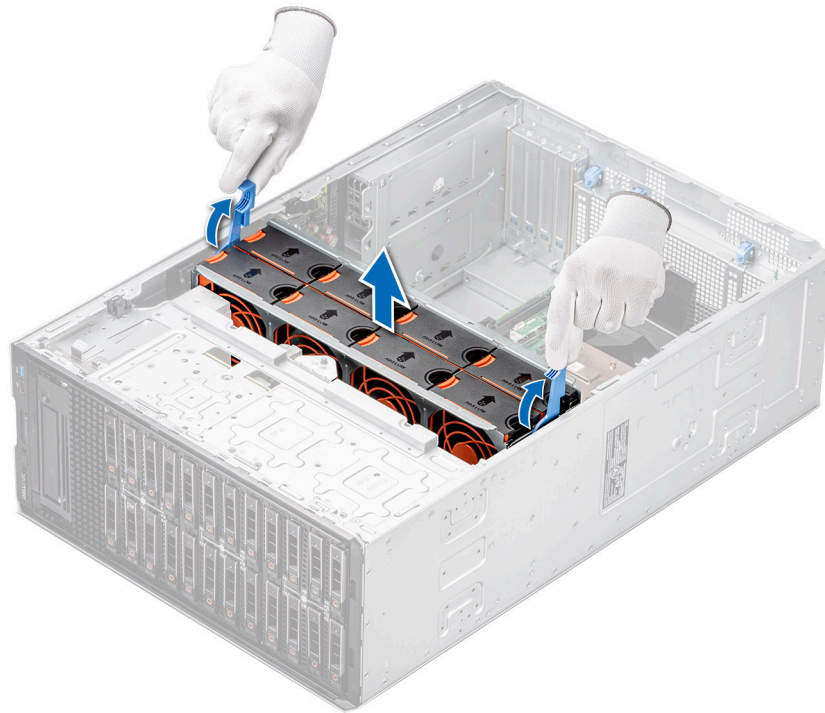
Figure 37. Removing the cooling fan cage
