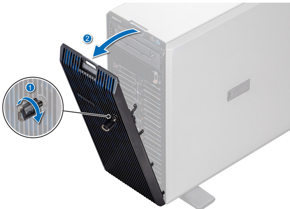
Figure 27. Removing the front bezel
