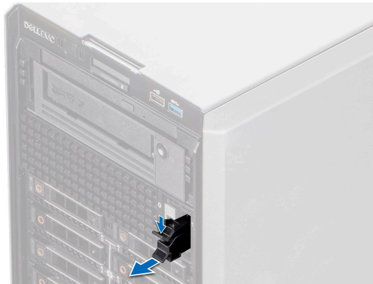
Figure 118. Removing the BOSS S2 card carrier blank
