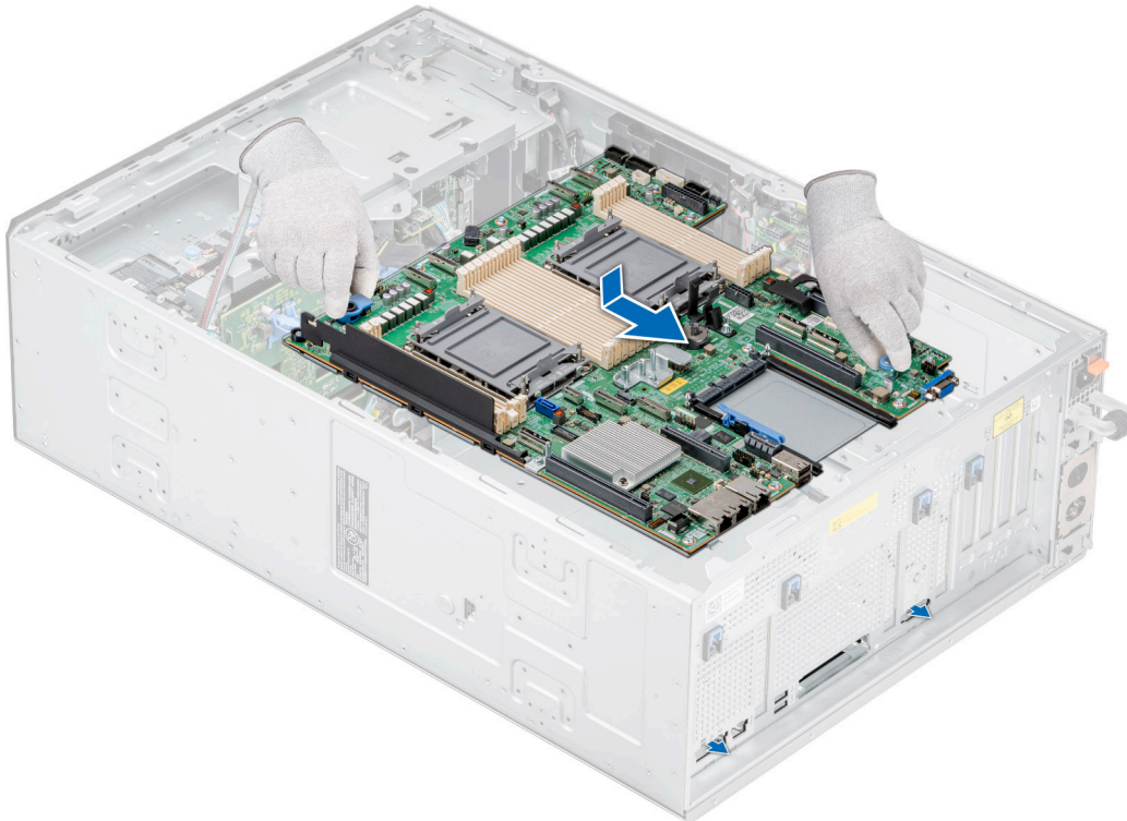
Figure 179. Installing the system board
