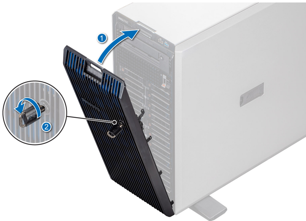
Figure 28. Installing the front bezel
