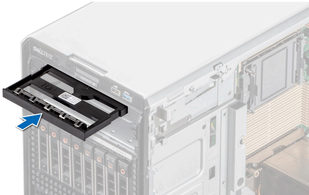
Figure 96. Installing the optical drive blank
