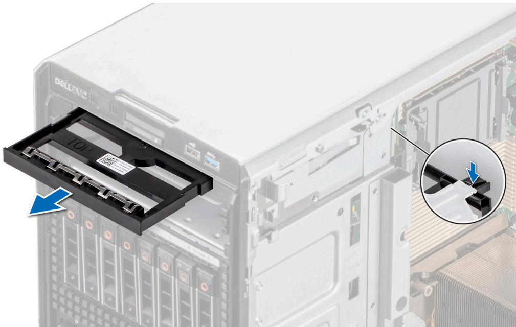
Figure 95. Removing the optical drive blank
