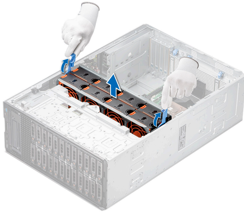
Figure 39. Removing the cooling fan cage
