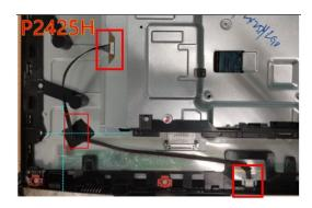
Star off 3 conductive tapes from "Main Shielding and "Panel"
