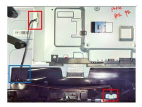
S12Tear off a long tape from "LVDS FFC"Disassemble "LVDS FFC" from "Panel"Take off "Main Shielding" from "Panel"
