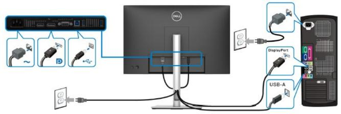
Connect/ disconnecting the HDMI cable (optional), USB 3.2 upstream cable and Power cable
