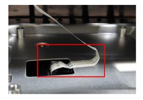
S6 Unlock 3 screws to disassemble "Control board" from "Rear Cover"
