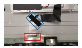
S8 Insert "Backlight wire" to "Panel" and "Power Board"
