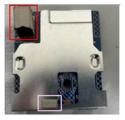
S10 Disassemble "USB board" from "USB Shielding"
