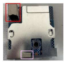
S11 Assemble "USB board" with "Middle Frame"
