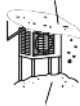
Install the unit high enough off the ground to prevent burying in snow
