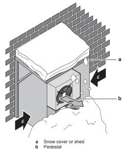
Prevailing wind direction С d Air outlet
