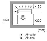
Allow 300 mm of work space below the ceiling surface and 250 mm for piping and electrical servicing.
