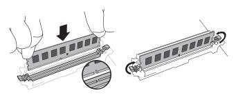
Using firm, even pressure, push DIMM into slot until clips snap into place. Do not assist clips.
