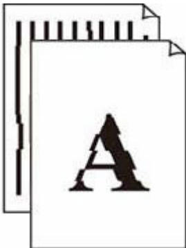
Lines Are Misaligned/Distorted
