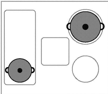
Boiling behavior may vary depending on the pot types, size of the pot and size of the cooking zone. For a more homogenous boiling behavior, a one step larger cooking zone might be used. To use a larger cooking zone does not cause wasting of energy at induction hobs, because the heat is only created in the relevant pot area.
