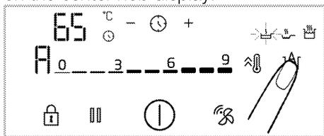
2. On the timer display, "65" is displayed as the lowest temperature setting for the setting of low temperature. By touching the  $\pm$  keys, you may change the temperature setting by increasing or decreasing it with 5 degrees increments.
