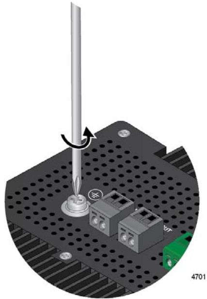
Figure 35. Loosening the Grounding Screw
