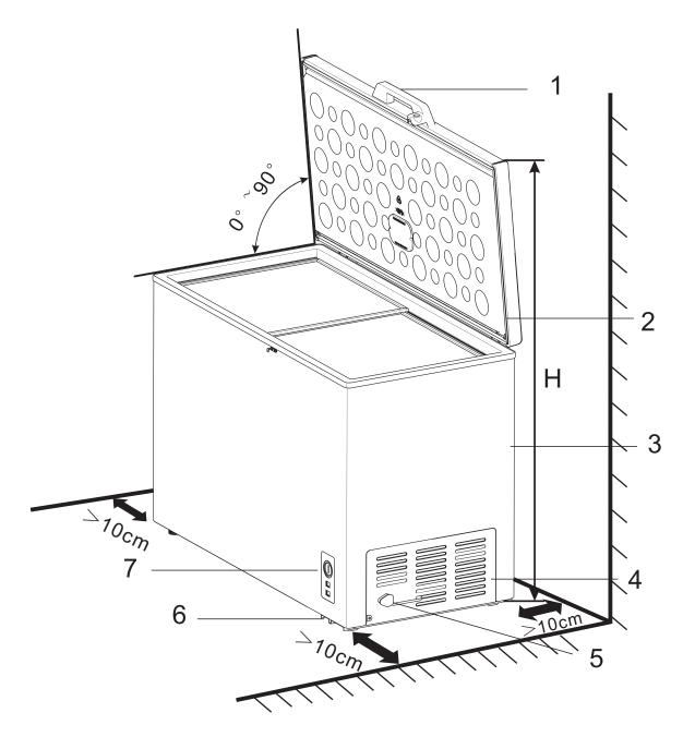
1. Door2. Door frame3. Cabinet4. Ventilation grid5. Power cord6. Wheel7. Thermostat
