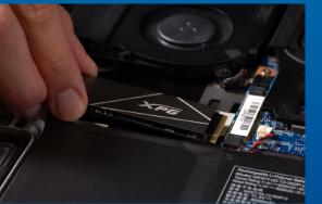
Use your small Phillips screwdriver to remove the screws on the motherboard. Align the notches in the SSD with the ridges in the PCIe slot, then insert at a an angle. Give it a final push to ensure it is securely in place.
